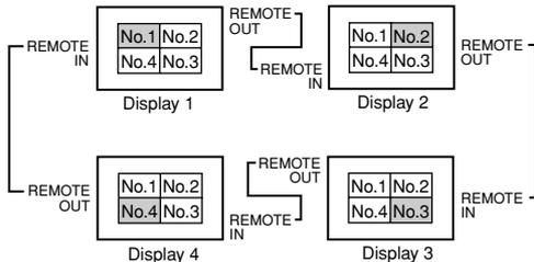
\* With the 3x3 video wall, connect the final display to the first display the same way as with 2x2 video wall.
